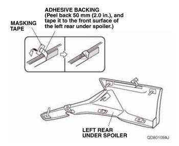
15. Install four seals and install the left rear under spoiler to the rear bumper as shown.
