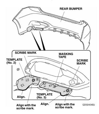
8. Using a pushpin, pierce the center of three scribe marks on the templates. Then remove the templates.
