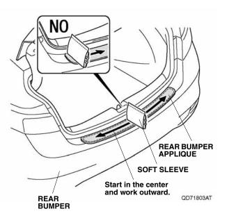
10. Slowly remove the protective film from the top of the rear bumper applique. Remove the protective film by pulling it slowly and horizontally; do not pull it vertically.
