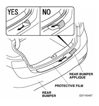
11. Repeat step 8 for the center of the rear bumper applique lower section.
