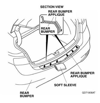
Using a shop towel, wipe away the excess 3M Protective Tape Application Solution. Allow the rear bumper applique to dry thoroughly.
