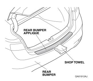
14. Remove the masking tape attached in step 2.
