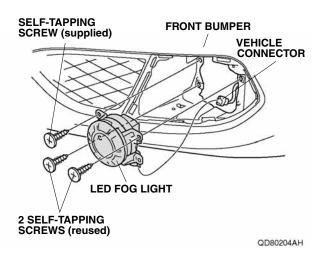
62. Reinstall the left fog light cover to the front bumper, and tighten one self-tapping screw.
