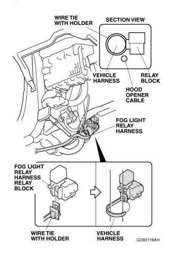
39. Unclip the vehicle connectors from the vehicle panel.
