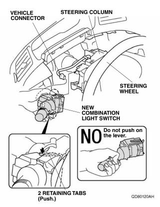
52. Plug the vehicle connector to the new combination light switch. Make sure the vehicle harness has some slack.
