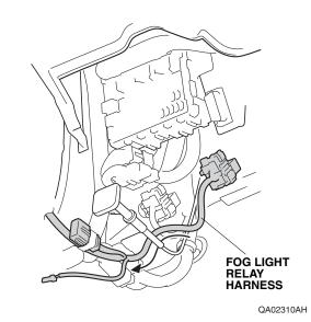
38. Attach the wire tie with holder to the fog light relay harness relay block, and secure it to the vehicle harness with the wire tie with holder. Do not secure the fog light relay harness relay block to the hood opener cable.
