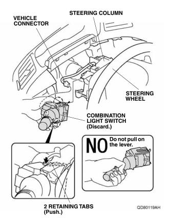
50. While pushing the two retaining tabs, slide the combination light switch out and remove it from the steering column.
