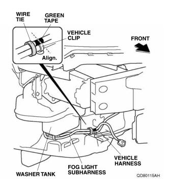
35. With the help of an assistant, plug the fog light subharness 4-pin connector into the fog light harness 4-pin connector. Install the front bumper and replug the vehicle connector. Securely install all clips.
