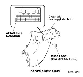
55. Attach the fuse label to the driver's kick panel.
