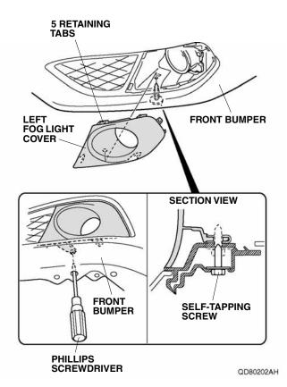
60. Remove the left fog light from the front bumper and unplug the vehicle connector.
