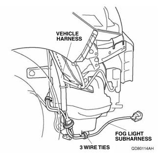
34. Align the green tape on the fog light subharness with the vehicle clip as shown, and secure the fog light subharness to the vehicle harness with one wire tie.
