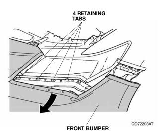
• With the help of an assistant, remove the front bumper. Place the front bumper on a blanket to prevent damage.
