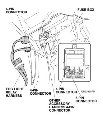
48. Secure the fog light relay harness to the vehicle harness with three wire ties.
