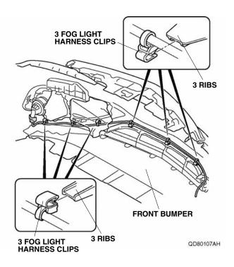
24. Plug the fog light harness 2-pin connector into the LED fog light.
