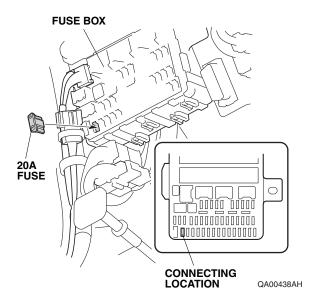
54. Using isopropyl alcohol on a shop towel, thoroughly clean the area where the fuse label will attach.
