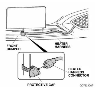
33. Secure the heater harness to the front bumper with a black wire tie.
