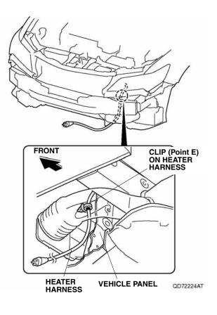
26. Secure the heater harness to the vehicle panel with a black wire tie.
