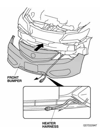
32. Attach the protective cap to the front bumper, and plug the heater harness connector into the protective cap.
