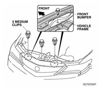
Remove the two self-tapping screws, two bolts, two short clips, and twelve medium clips.
