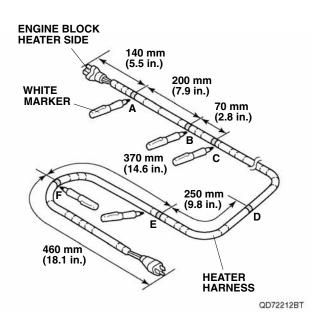
9. Install one wire tie with clip to the heater harness at point E.
