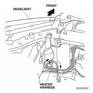
25. Secure the clip (point E) on the heater harness to the vehicle panel.
