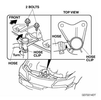
11. Rotate the coolant hose clip as shown.
