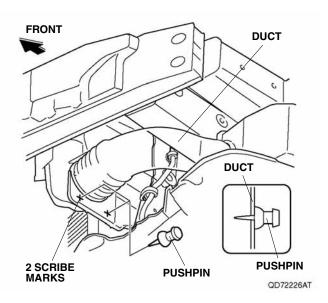
28. While wearing eye protection, drill the two pierced marks with a 3 mm drill bit, then enlarge the holes with a 5 mm drill bit. Remove any burrs.
