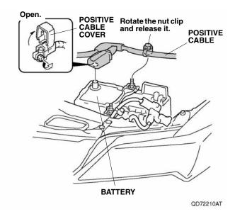
7. Remove the battery, the plate, and the covers.
