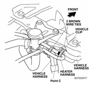
19. Secure the heater harness to the vehicle harness with one brown wire tie.
