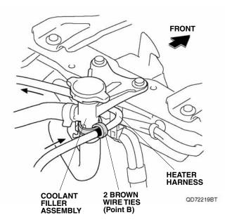
18. Align the heater harness white mark (point C) with the vehicle clip, secure the heater harness to the vehicle harness with a brown wire tie.
