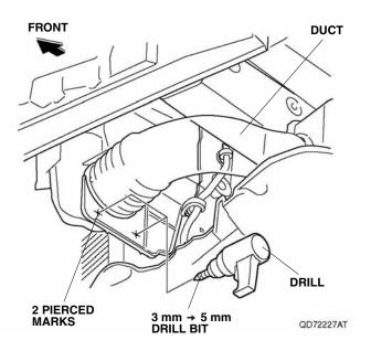
29. Secure the heater harness to the duct with one black wire tie.
