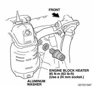
14. Plug the connector end of the heater harness into the engine block heater. Make sure the heater harness connector is fully seated in the engine block heater.
