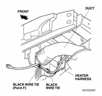
30. Secure the heater harness to the duct with one black wire tie at the white mark (point F).
