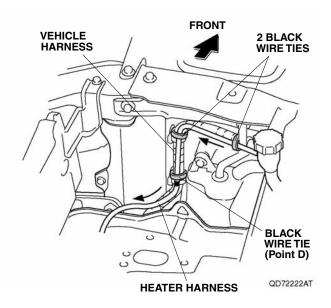
23. Secure the heater harness to the vehicle harness with a black wire tie at the white mark (point D).
