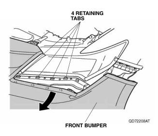
• With the help of an assistant, remove the front bumper and unplug the vehicle connector. Place the front bumper on a blanket to prevent damage.
