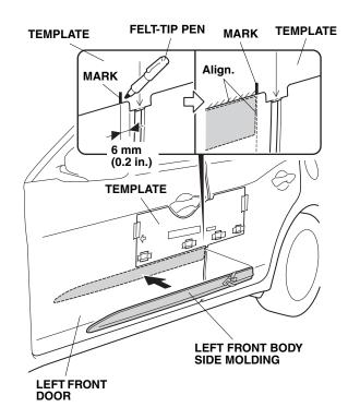
6. Align the left front body side molding with the template and the mark on the template, then attach it to the left front door as shown. Go to step 8.
