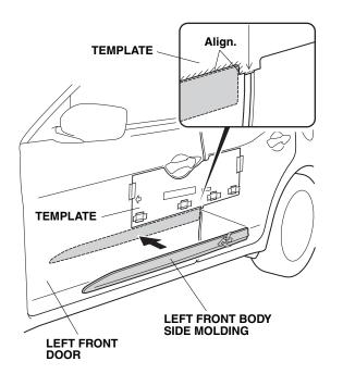
8. Press on the left front body side molding firmly with the palm of your hand while removing about 50 to 100 mm (2.0 to 3.9 in.) of the adhesive backing at a time.
