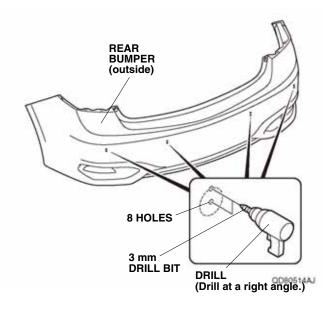
38. While wearing eye protection, and drilling from outside of the rear bumper, enlarge the two outer 3 mm lower holes to 24 mm using a 24 mm hole saw. NOTE: Make sure to drill at a right angle to the rear bumper. Remove any burrs.
