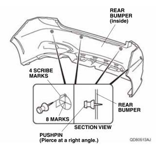
37. While wearing eye protection, drill the eight pierced marks with a 3 mm drill bit from outside of the rear bumper.
