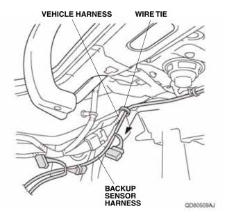
22. Unplug the vehicle 28-pin connector, and plug it into the backup sensor harness 28-pin connector. Plug the remaining backup sensor harness 28-pin connector into the vehicle 28-pin connector.
