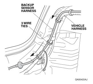
32. Remove the vehicle ground bolt. Attach the backup sensor harness ground terminal to the vehicle ground terminal, and reinstall the vehicle ground bolt.
