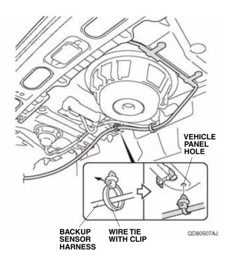
20. Secure the backup sensor harness with the two wire ties with clip as shown. If there is a vehicle harness, cut off the clips of the two wire ties with clip and secure the backup harness to the vehicle harness.
