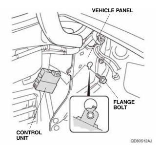
28. Route the backup sensor harness as shown. Plug the backup sensor harness 14-pin connector into the control unit.
