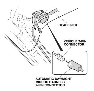
24. Plug the vehicle 2-pin connector into the automatic day/night mirror harness 2-pin connector.
