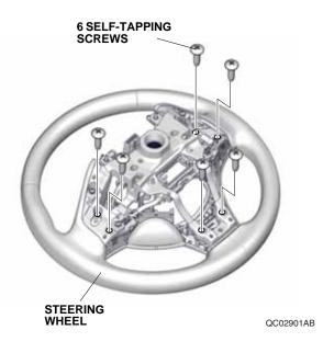
13. Remove the switch assembly and cable guide.
