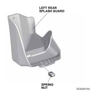
9. Loosely install the left rear splash guard on the left bracket and left rear inner fender with one 5 x 20 mm self-tapping screw and two of the self-tapping screws removed in step 1.
