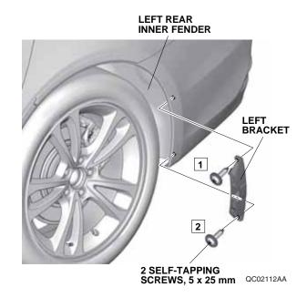
6. Secure the left bracket to the rear bumper using a 5 x 25 mm self-tapping screw. Thread the screw into the spring nut through the left rear inner fender.
