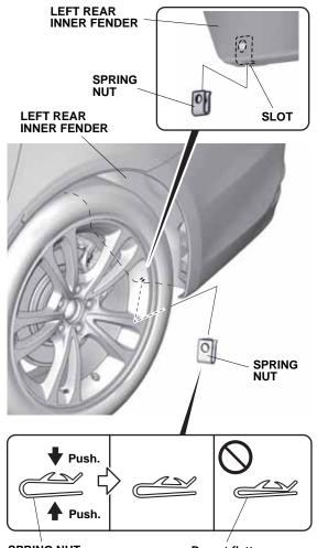
SPRING NUT (Compress slightly before install.)
