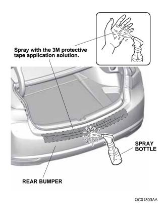
3. Remove the adhesive backing from the side of the rear bumper applique with the 3M mark.
