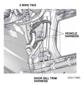
31. Secure the door sill trim harness to the vehicle harness with two wire ties.
