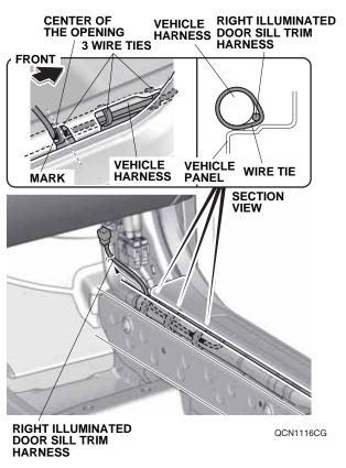
25. Secure the right illuminated door sill trim harness to the vehicle harness with three wire ties as shown.
