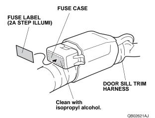
27. Locate the vehicle 2-pin connector. Remove the tape and disconnect the dummy connector.
