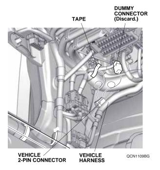
13. Plug the vehicle 2-pin connector into the door sill trim harness 2-pin connector.
