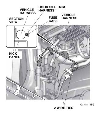
16. Secure the door sill trim harness to the vehicle harness with two wire ties.
