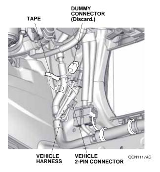
28. Plug the vehicle 2-pin connector into the door sill trim harness 2-pin connector.
