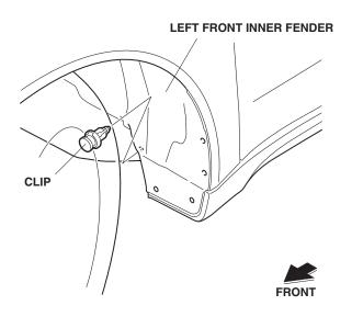
4. Install the left front splash guard to the left front inner fender with two self-tapping screws and the clip removed in step 3.
