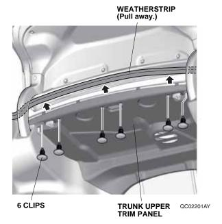
Pull down the trunk upper trim panel. Push the tab, then pull down the right seat-back release lever to release the hook and remove the lever. Remove the left seat-back release lever the same way.
