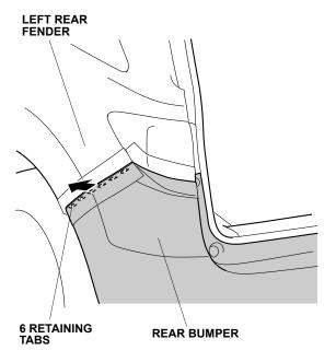
Release one retaining tab on each side.
