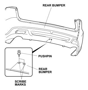
5. While wearing eye protection, drill the two pierced marks with a 3 mm drill bit, then enlarge the holes with a 20 mm hole saw.
