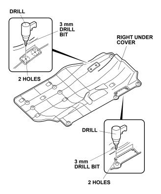
11. Enlarge two holes made in the right under cover in step 10 with a 10 mm drill bit.
