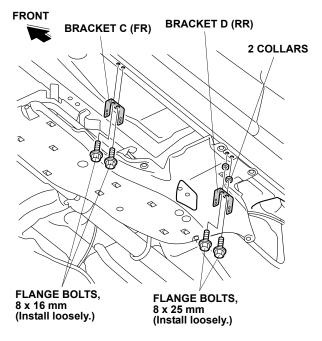
16. Secure a bracket D (RR) to the vehicle panel with two collars and two loosely-installed 8 x 25 mm flange bolts.
