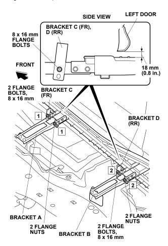
24. Visually check that the left running board is installed parallel to the vehicle.
