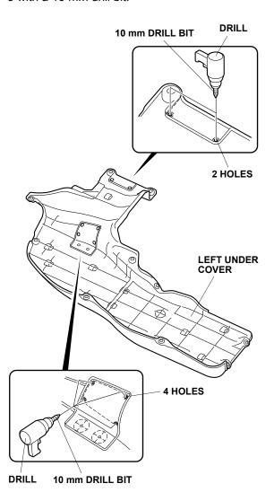
7. Enlarge two holes made in the left under cover in step 5 with a 30 mm hole saw. Remove any burrs.
