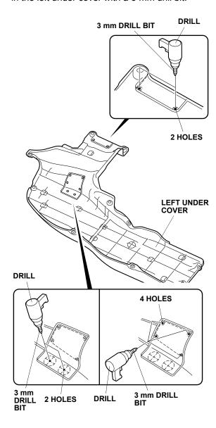
6. Enlarge six holes made in the left under cover in step 5 with a 10 mm drill bit.
