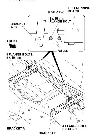
Adjust the position of the running board as shown. Tighten the four 8 x 16 mm flange bolts and four flange nuts loosely installed in step 18 in the order 1→2. Torque the flange bolts to 22 N·m (2.2 kgf·m, 16 lbf·ft).
