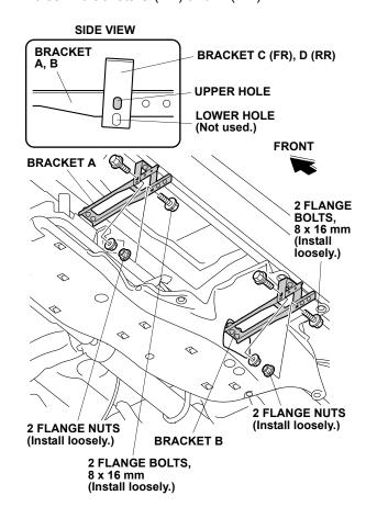
19. Secure the left running board to bracket A and bracket B with eight loosely-installed 8 x 16 mm flange bolts.
