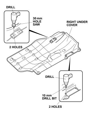
12. Enlarge two holes made in the right under cover in step 10 with a 30 mm hole saw. Remove any burrs.
