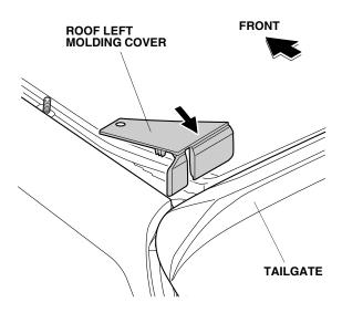
16. Install the purple clip removed in step 12 to the roof left molding.
