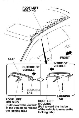
Place a blanket over the roof of the vehicle under the mark on the roof left molding. Be careful not to deform the roof left molding when measuring and cutting.
