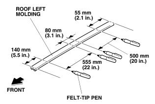
14. While wearing eye protection, use an air saw to cut the roof left molding at the marks made in step 13.
