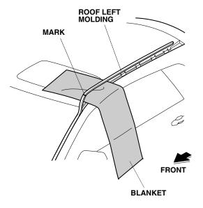
8. Place an empty cardboard box (approx. 120 mm tall) under the roof left molding near the mark.
