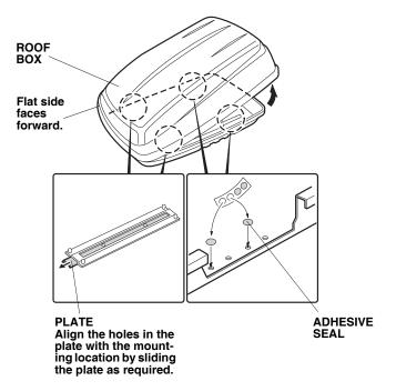
3. Attach an adhesive seal over each of the four unused mounting holes (two on each side) at the rear of the base of the box. The seals will help prevent water from entering the roof box. Then, remove the roof box from the crossbars.
