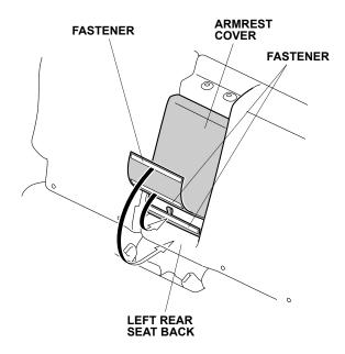
6. Secure the fastener to the bottom of the left rear seat back.
