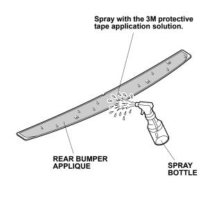
8. Align the v-notch on the rear bumper applique to the mark on the masking tape, and align the edge along the crease of the curved surface as shown. Smooth the rear bumper applique along the rear bumper.
