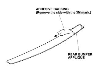
7. Spray the rear bumper applique with the 3M protective tape application solution.
