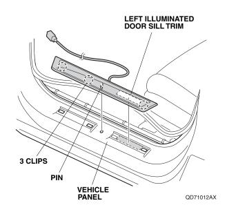
21. Using isopropyl alcohol on a shop towel, thoroughly clean the vehicle panel where the protective tape will attach. Attach one piece of protective tape to the vehicle panel as shown.
