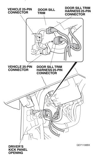
36. Plug the remaining door sill trim harness 25-pin connector into the vehicle 25-pin connector.
