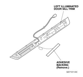
20. Install the left illuminated door sill trim to the vehicle panel with three clips. Using the palm of your hand, firmly press the left illuminated door sill trim against the vehicle panel.
