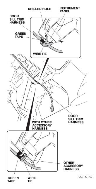
43. Secure the door sill trim harness to the vehicle frame with two wire ties as shown. If the vehicle is already equipped with other accessory harness, secure the door sill trim harness to the other accessory harness with one wire tie as shown.
