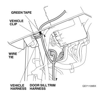
Secure the door sill trim harness and the 25-pin connectors to the vehicle harness with two wire ties.
