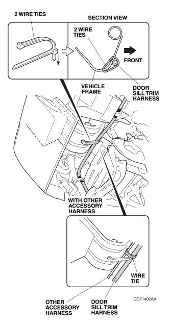
44. Attach one wire tie with clip around the green tape on the door sill trim harness, then secure the harness to the hole in the vehicle frame with the clip. If the vehicle is already equipped with other accessory harness, secure the door sill trim harness to the other accessory harness with one wire tie as shown.
