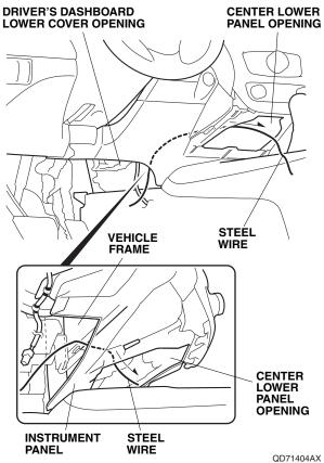
46. Route the steel wire from the center lower panel opening to the glove box opening.
