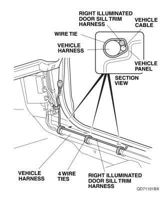
26. Route the left illuminated door sill trim harness along the vehicle harness, and secure it to the vehicle harness with four wire ties.
