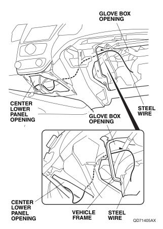
47. Attach the steel wire to the door sill trim harness with electrical tape.
