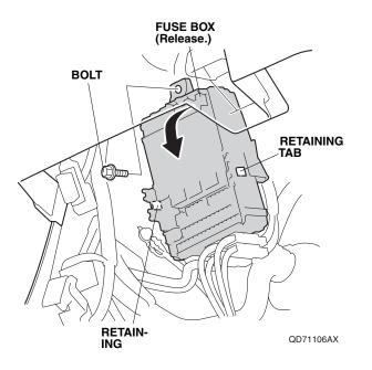
31. Using isopropyl alcohol on a shop towel, thoroughly clean the fuse case where the fuse label will attach. Attach the fuse label (2A STEP ILLUMI) to the fuse case on the door sill trim harness.
