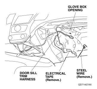
49. Secure the door sill trim harness to the vehicle harness with one wire tie.
