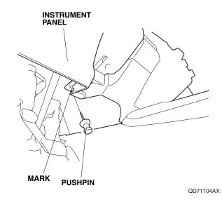
29. While wearing eye protection, drill the pierced mark with a 3 mm drill bit, then enlarge the hole with a 6 mm drill bit. Remove any burrs.To prevent drilling through the inner panel, wrap tape around the drill bit 10 mm (0.39 in.) away from the tip
