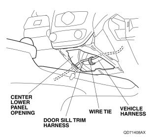
50. Route the door sill trim harness along the vehicle harness, and secure it to the vehicle harness with four wire ties.
