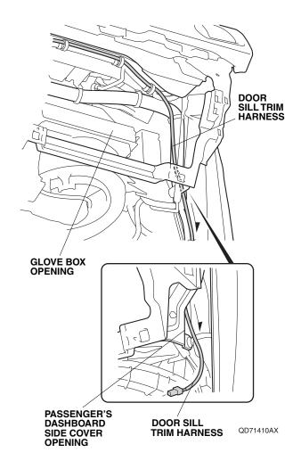
52. Plug the door sill trim harness 2-pin connector into the right illuminated door sill trim harness 2-pin connector.
