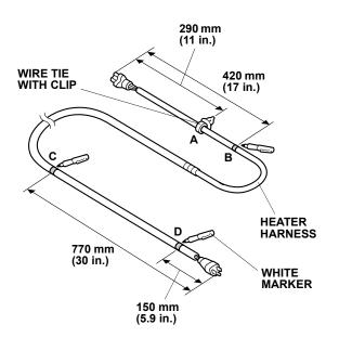
15. Using a white marker, mark the heater harness at the three measurements shown.
