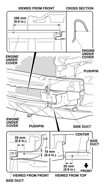
While wearing eye protection, drill the three pierced marks on the side duct and engine under cover with a 3 mm drill bit, then enlarge the three holes with a 7 mm drill bit. Remove any burrs. Wrap tape around each drill bit 7 mm away from the tip or use a drill stop.
