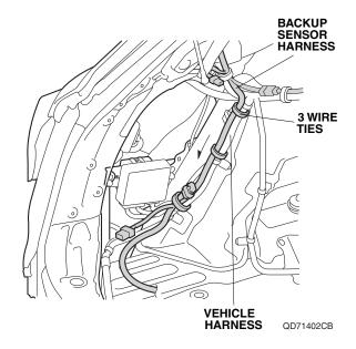
32. Plug the backup sensor harness 14-pin connector into the control unit.
