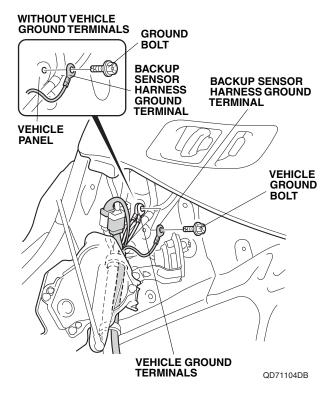
25. Secure the backup sensor harness ground terminal to the vehicle ground terminals with the vehicle ground bolt just removed. Do not put the ground terminal calkings on top of one another.
