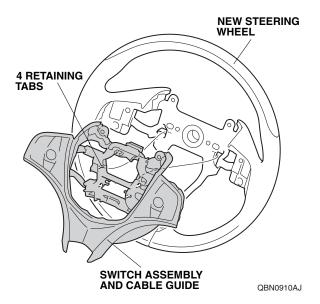
16. Secure the switch assembly and cable guide to the new steering wheel with the six self-tapping screws.
