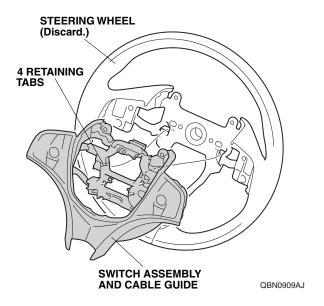
15. Install the switch assembly and cable guide to the new steering wheel.
