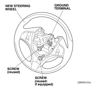
18. Install the left and right paddle shifters to the new steering wheel with four screws.
