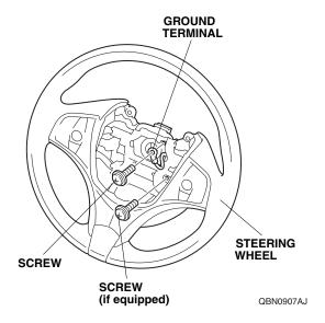
13. Remove the six self-tapping screws.
