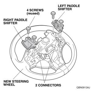
19. Plug two connectors into the left and right paddle shifters.
