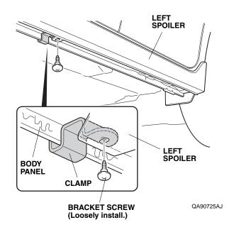
36. Assemble the one screw and the one washer-nut.
