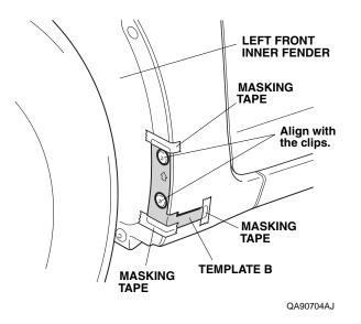
10. Using a felt-tip pen, mark the left front fender at the area shown.
