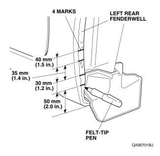
6. Using a utility knife, remove the undercoating in the areas shown.
