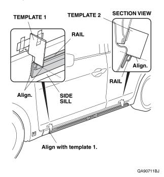
20. While holding the rail in place, slowly and carefully remove each adhesive backing.
