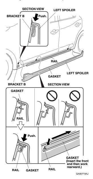
27. Lightly tap the left spoiler to remove any gap between the left spoiler and the left rear fenderwell.
