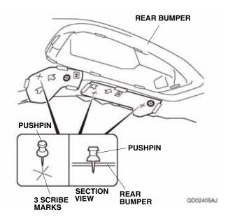
9. Using a pushpin, pierce the center of four scribe marks on the rear bumper.
