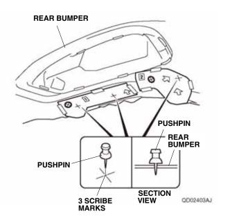
Turn the template No. 2 over, and align the templates No. 2 and No. 3 with the rear bumper as shown.
