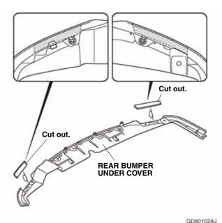
5. Align the templates No. 1 and No. 2 with the rear bumper as shown. Attach the templates to the rear bumper using masking tape.
