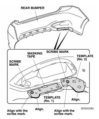
6. Using a pushpin, pierce the center of three scribe marks on the templates. Then remove the templates.
