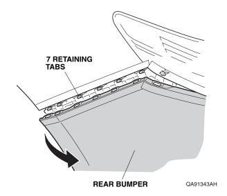
• Release the two retaining tabs on each side.
