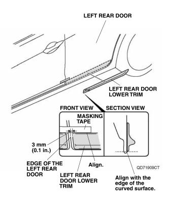
12. While applying light pressure to the rear door lower trim, carefully remove the two adhesive backings. Using the palm of your hand, firmly press the left rear door lower trim onto the left rear door.
