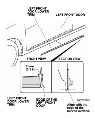
5. While applying light pressure to the front door lower trim, carefully remove the two adhesive backings. Using the palm of your hand, firmly press the left front door lower trim onto the left front door.
