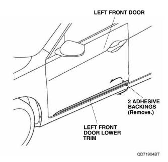
6. Using a rubber roller, apply firm pressure, especially at the ends to set the adhesive.
