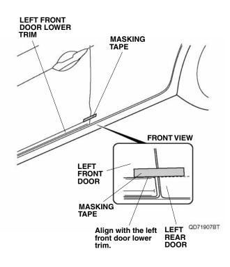
9. Peel back the ends of two adhesive backings on the left rear door lower trim and attach them to the front of the trim with masking tape.
