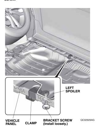
43. Assemble one screw and one washer-nut.
