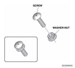
44. Tighten the screw into the clamp securely, then finger tighten the washer-nut against the clamp. While holding the screw, tighten the washer-nut 90° clockwise.
