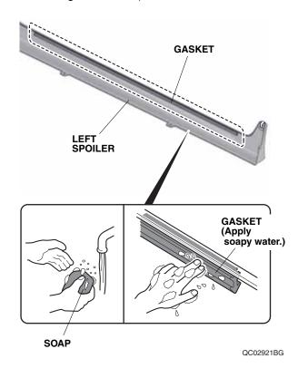
25. Secure the hook on the spoiler to the bracket and align the gasket on the spoiler with the rails. Insert the rear part of the gasket into the rail first, then work forward. Move the spoiler up and down gently to make sure that the gasket is installed securely to the rails.
