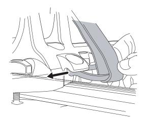
7. Rotate the buckle up to lock it into the base. Repeat this step for the remaining bases.
