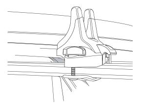
6. Slide the buckle on the attachment strap into the clip on the base.
