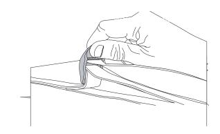
2. Rotate the buckle down to unlock the attachment straps, and slide the buckles out of the bases.
