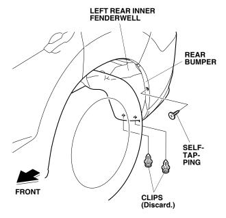
7. Remove and discard the two clips from the left rear inner fenderwell.
