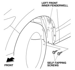
4. Install the left front splash guard to the left front inner fender with two washer-screws and the two self-tapping screws removed in step 3. Tighten in the order 1→2→3→4.
