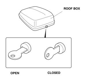
**Locking:** Press down on the lid. There should be an audible click. Be sure the lid is latched by attempting to lift the lid. Turn the key clockwise to lock the roof box. Remove the key while not in use. Be sure the straps do not dangle from the box.
