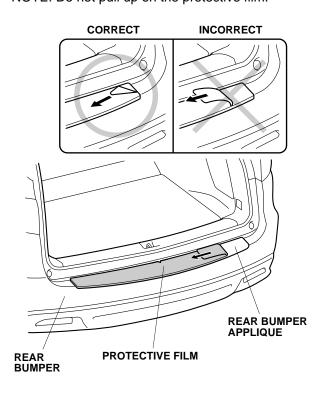
13. Repeat step 10 at the center of the lower section of the rear bumper applique.
