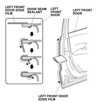
tape application solution. NOTE: Spray only the outer surface.
