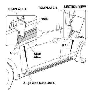
20. While holding the rail in place, slowly and carefully remove each adhesive backing.
