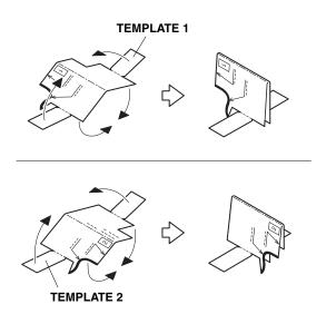
15. Insert the tab on template 1 into the gap between the left front door and the side sill at the measurement shown. With the template flush against the side sill, tape the template to the door. There should be no gap between the template and the side sill.
