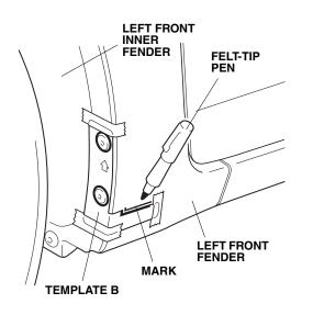
11. Carefully remove template B. Do not damage the template, it is needed to mark the right side of the vehicle.
