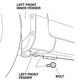
3. Using a utility knife, remove the undercoating in the area shown.
