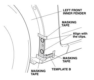
10. Using a felt-tip pen, mark the left front fender at the area shown.
