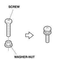
37. Install the screw into the clamp and tighten it securely. Then finger-tighten the washer-nut against the clamp. While holding the screw, tighten the washer-nut.
