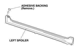
26. Insert the bracket on the spoiler into bracket B, and align the gasket on the left spoiler with the rail. Insert the front end of the gasket into the rail first, then work rearward. Move the left spoiler gently up and down, while checking that the gasket is installed securely in the rail.
