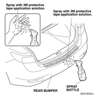
4. Remove the adhesive backing (side with the 3M mark) from the rear bumper applique.
