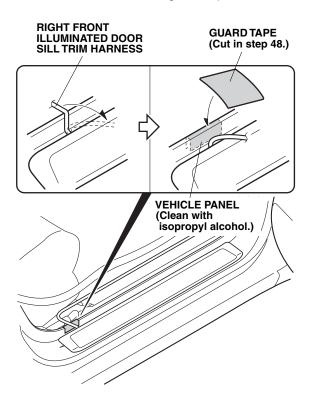
73. Attach one cut piece of guard tape to the vehicle panel in the area shown.
