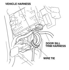
24. Secure the door sill trim harness to the vehicle harness with two wire ties.
