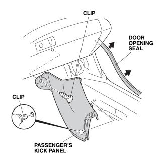
4. Pull away the door opening seal from around the passenger's dashboard side cover.
