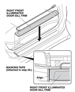
70. Attach the right front illuminated door sill trim to the vehicle panel by removing the three adhesive backings and pressing on the trim firmly with your hands.
