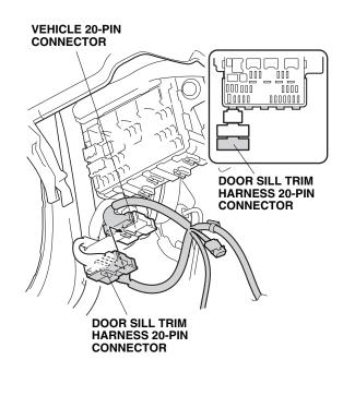
21. Attach the clip on the door sill trim harness to the fuse box.
