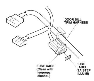
18. Attach the fuse label to the door sill trim harness fuse case.
