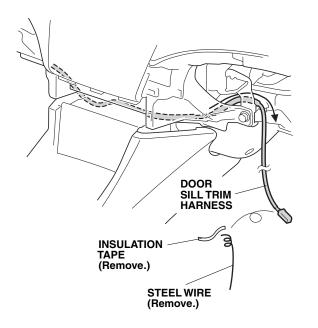
30. Remove the steel wire from the door sill trim harness.
