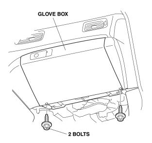
16. Remove the glove box (three self-tapping screws and unplug the vehicle connectors).
