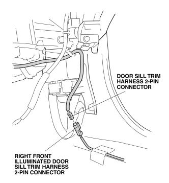
81. Secure the door sill trim harness 2-pin connector to the vehicle harness with one wire tie.
