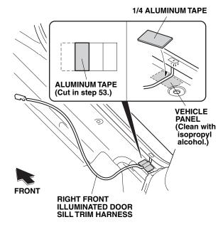
76. Secure the right front illuminated door sill trim harness to the vehicle panel with one cut piece of aluminum tape.
