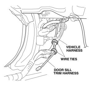
25. Secure the door sill trim harness to the vehicle harness with one wire tie.
