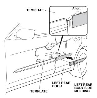
12. Press on the left rear body side molding firmly with the palm of your hand while removing about 50 to 100 mm (2.0 to 3.9 in.) of the adhesive backing at a time.
