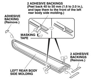
11. Align the left rear body side molding with the template, and attach it to the left rear door as shown.
