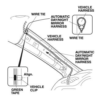
22. Secure the automatic day/night mirror harness to the vehicle harness with three wire ties as shown.
