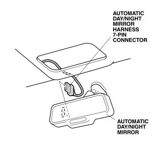
27. Route the automatic day/night mirror harness through the groove in the harness cover. Secure the harness cover to the mirror stay. Slide the harness cover behind the headliner.
