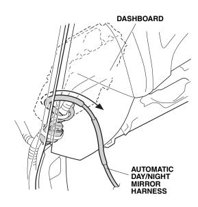
20. Insert the automatic day/night mirror harness between the dashboard and the driver's A-pillar.
