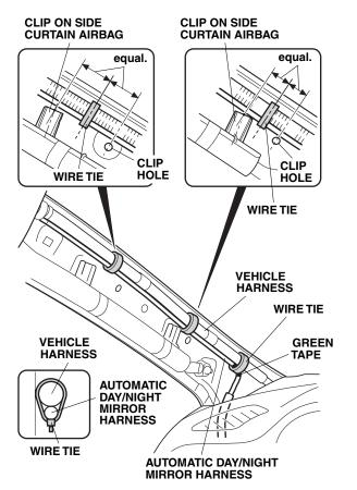
23. Pull the two automatic day/night mirror harness 2-pin connectors out through the hole in the headliner as shown. Be careful not to crease the headliner.
