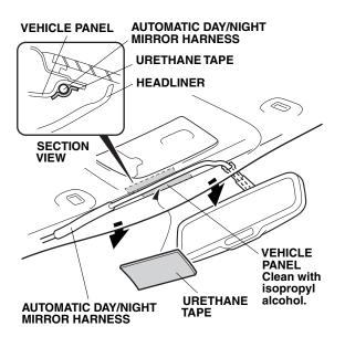
29. Secure the automatic day/night mirror harness to the vehicle panel with one urethane tape as shown. Be careful not to crease the headliner.
