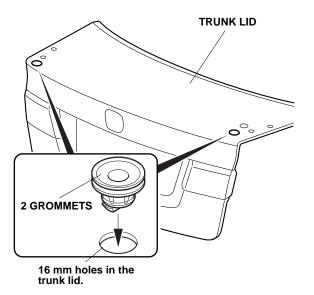
17. Open the trunk lid and position the wing spoiler on the trunk lid as shown. Seat the wing spoiler harness grommet into the hole as shown, and loosely install the wing spoiler using the two cap nuts.
