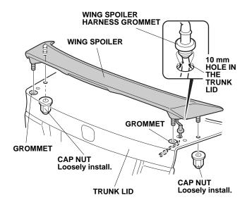
18. Install a 6 x 12 mm washer screw into each side of the wing spoiler.
