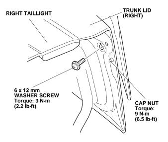
19. Torque the washer-screw to 3 N·m (2.2 lb-ft) then torque the cap nuts to 9 N·m (6.5 lb-ft). Reinstall the rubber stop you removed in step 9.
