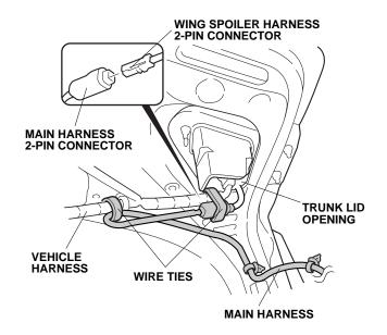
23. Secure the main harness to the vehicle harness using two wire ties.
