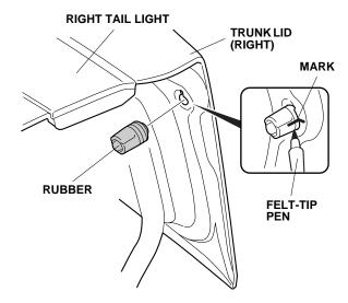
On the inside of the trunk lid, locate the identification mark on the trunk lid. Lightly center-punch the mark. Repeat on the left side of the trunk lid.
