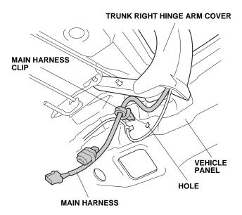
31. Unplug the vehicle 4-pin connector from the right taillight, and plug the main harness 4-pin connector into the taillight. Plug the taillight 4-pin connector into the main harness 4-pin connector.
