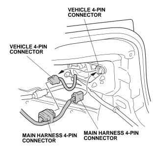
32. Secure the main harness to the vehicle harness using two wire ties. If the vehicle you are working on does not have a harness, secure the main harness to the hole in the vehicle as shown.
