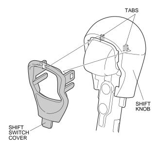
4. Remove the two screws from the shift knob, and remove the shift knob by pulling it up.
