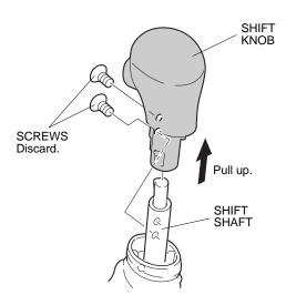
5. Install the select knob using the two new screws. Using a Torque screwdriver, torque the screws to 1.57 N·m (14 lb-in) Do not overtighten the screws.
