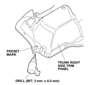
7. Install one 6 x 16 mm hex bolt, spring washer, plain washer, and T-anchor through the hole you just made. Tighten securely.
