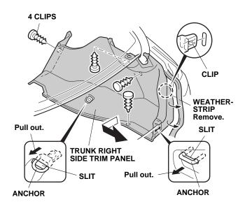
5. On the inside of the trunk right side trim panel, locate the preset mark in the location shown. Using a pushpin, pierce the center of the preset mark.
