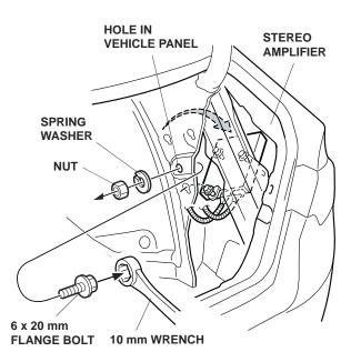
9. Locate the hole in the vehicle panel. Install one 6 x 20 mm flange bolt through the vehicle panel hole, then install a spring washer and nut. Reinstall the stereo amplifier.
