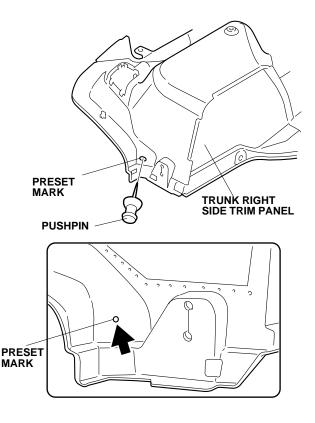
6. While wearing eye protection, drill the pierced mark to 6.5 mm. First drill with a 3 mm drill bit, and finish with a 6.5 mm drill bit.
