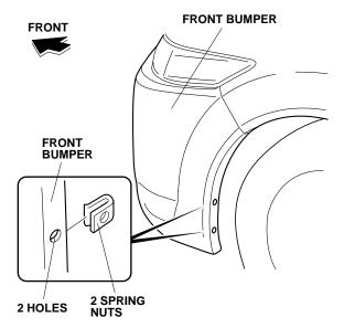
4. Install three clip nuts to the bottom of the front bumper as shown.
