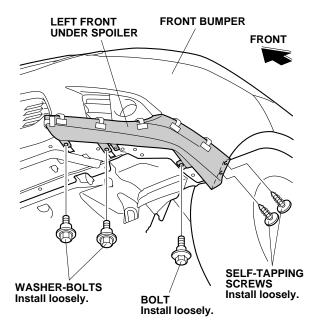
8. While applying light pressure to position the left front under spoiler, carefully remove the tabs.
