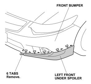
9. Using the palm of your hand, firmly press the left front under spoiler against the front bumper. Start at the back and work toward the front. Make sure there is no gap.
