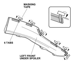
7. Loosely install the left front under spoiler to the front bumper with two washer-bolts, one bolt, and two self-tapping screws.
