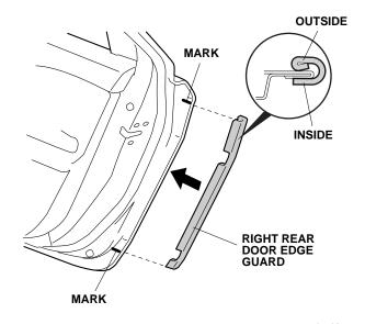
Using a rubber mallet, lightly tap around each bend in the right rear door edge guard.
