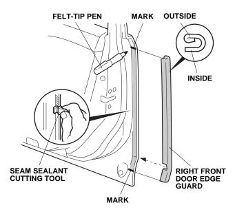
5. Position the cutting edge of the seam sealant cutting tool against the door edge, and trim the seam sealant from mark to mark.
