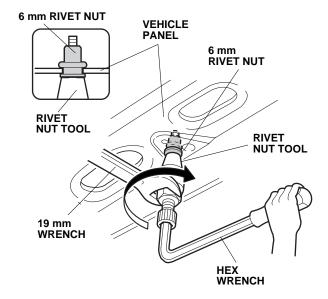
4. Remove the rivet nut tool from the 6 mm rivet nut by turning the hex wrench counterclockwise.
