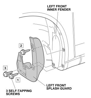
4. Turn the steering wheel clockwise, and repeat steps 2 and 3 to install the right front splash guard.
