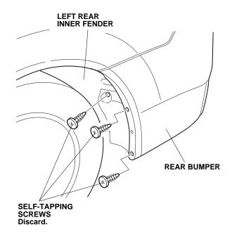
Secure the left rear splash guard to the left rear inner fender and rear bumper with three self-tapping screws in the order shown below.
