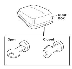
Locking: Press down on the lid. There should be an audible click. Be sure the lid is latched by attempting to lift the lid. Turn the key clockwise to lock the roof box. Remove the key while not in use. Be sure the straps do not dangle from the box.
