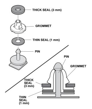
13. Install one pin grommet assembly into each slot in the trunk spoiler. Align the pins in each slot with the marks shown.
