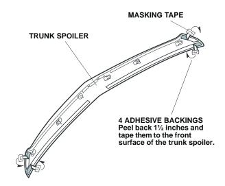
11. Using the alcohol pads supplied, clean the trunk lid where the trunk spoiler will be attached. Allow the alcohol to dry.
