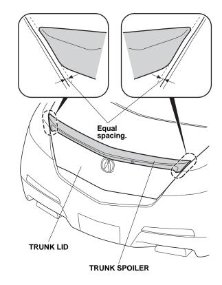
15. Install the trunk spoiler on the trunk lid using the three pins. Install the pins securely by applying pressure on the trunk spoiler with the palm of your hand. Listen carefully for each pin to click into place in its grommet.
