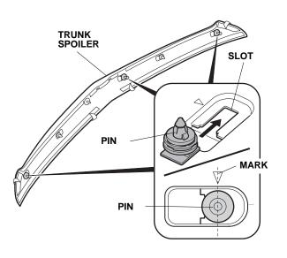
14. Center the spoiler on the trunk lid, and check the distance on each side.
