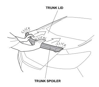
16. Open the trunk lid. Use a flashlight to confirm that the three pins are seated properly in their grommets.
