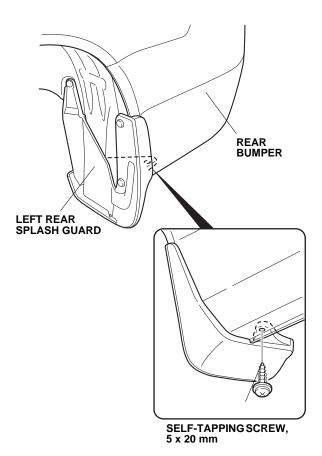
11. While holding the left rear splash guard against the rear bumper, tighten the four self-tapping screws in the order shown. Make sure there is no gap between the left rear splash guard and the vehicle. If there is, loosen the four self-tapping screws, adjust the splash guard to remove the gap, and retighten the screws.
