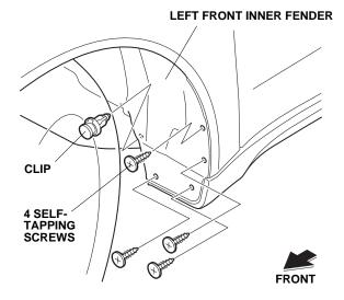
3. Loosely secure the left front splash guard on the left front inner fender with four self-tapping screws.
