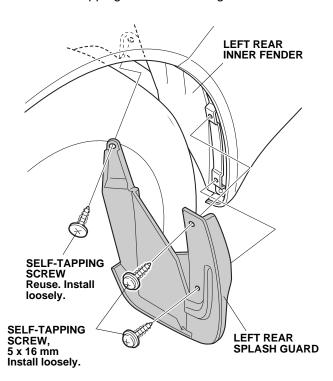
10. Secure the left rear splash guard to the rear bumper with a loosely-installed 5 x 20 mm self-tapping screw.
