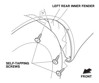
7. Secure the left bracket on the left rear inner fender with two self-tapping screws.
