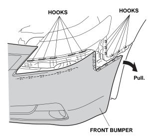
8. With the help of an assistant, remove the front bumper (unplug the five vehicle connectors). Place the front bumper on a blanket so it does not get damaged.
