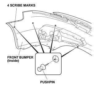
While wearing eye protection, drill the four pierced marks using a 3 mm drill bit, then finish with a 10 mm drill bit.
