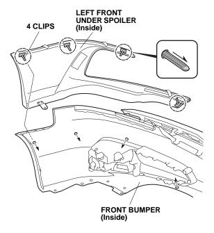
15. Secure the four clip holders onto the four clips.
