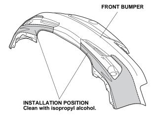
14. Install the left front under spoiler on the front bumper.
