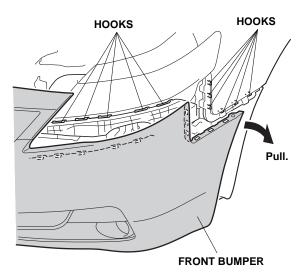
With the help of an assistant, remove the front bumper (unplug the five vehicle connectors). Place the front bumper on a blanket so it does not get damaged.
