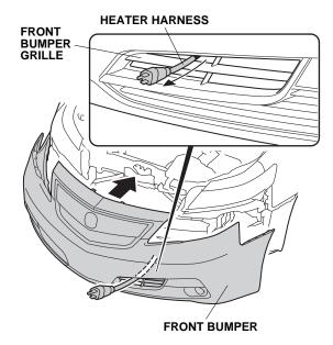
24. Secure the heater harness to the front bumper grille using one black wire tie.
