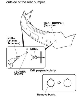
49. While wearing eye protection, use a 24 mm hole saw
