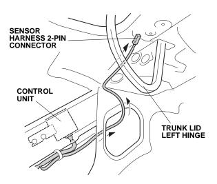
27. Plug the sensor harness 2-pin connector into the buzzer harness 2-pin connector.
