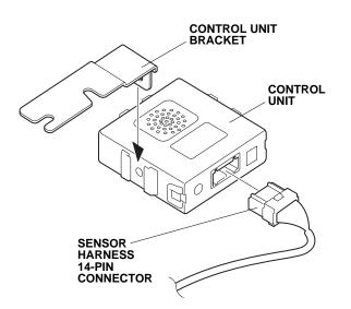
16. Plug the sensor harness 14-pin connector into the control unit.
