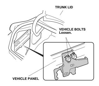
18. Slide the control unit bracket over the two vehicle bolts.
