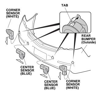
54. Install the four sensor clips.
