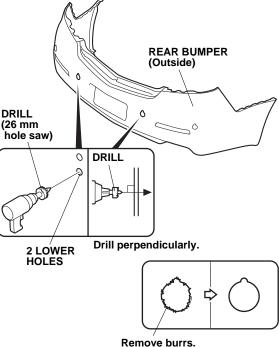
53. Install two center sensors (blue) and two corner sensors (white) into the rear bumper.
