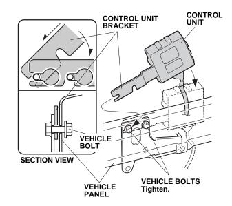
19. Tighten the two vehicle bolts.
