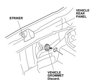
34. Route the sensor harness along the vehicle harness.
