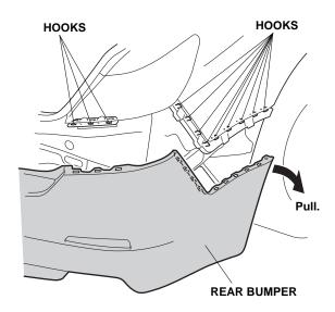
12. With the help of an assistant, remove the rear bumper (four hooks, and unplug the two vehicle connectors). Place the rear bumper on a blanket to prevent damage.
